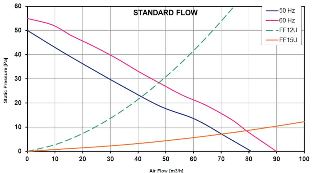
Curve characteristic of the filter fan and exhaust filter curves
